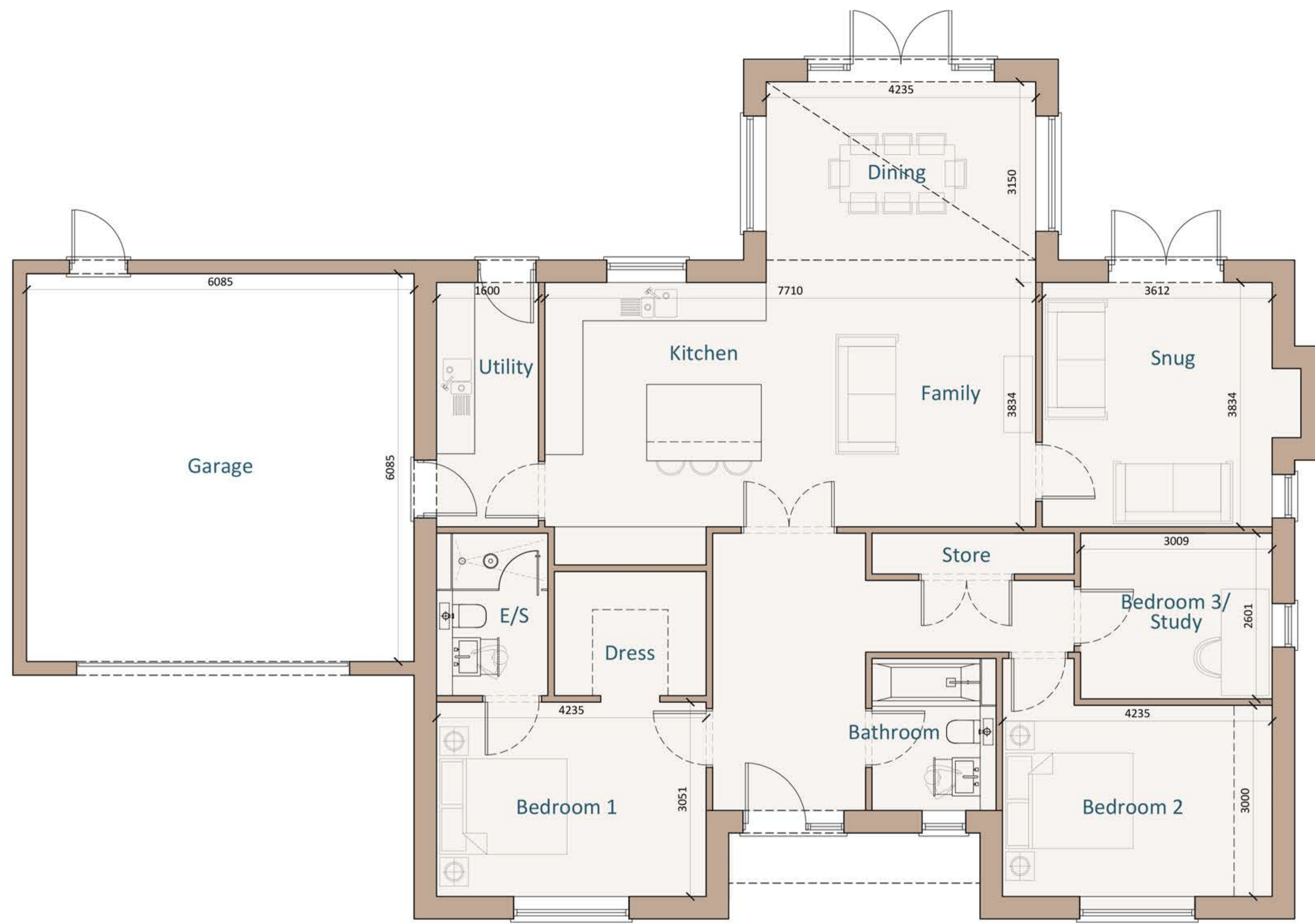
Proposed Ground Floor Plan Scale 1:50
